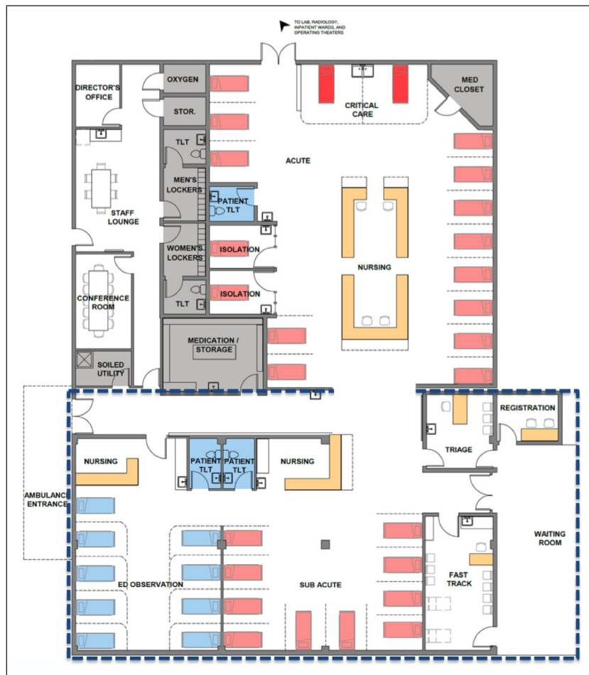
Figure 3: HUM ED Redesign. The dashed box indicates new construction, whereas the remainder of the space reflects redesign within the existing footprint of the HUM ED. Patients move from the waiting area to dedicated triage space into the appropriate fast-track, acute, sub-acute, or observation areas. Staff workspace is positioned to prioritize line-of-site to critical patients.
