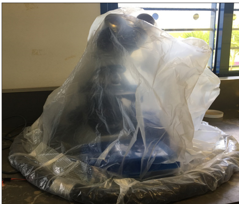
Figure 2: Humidity control system containing microscope.
